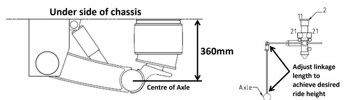
The ABS Trailquip dolly is designed for use with a ride height of 360mm. If the ride height on your dolly is not the same, it may affect the performance of the suspension and lead to premature failure of the suspension components. The ride height should be checked immediately and there after every 10,000kms to ensure the air suspension is working within its design limits.
