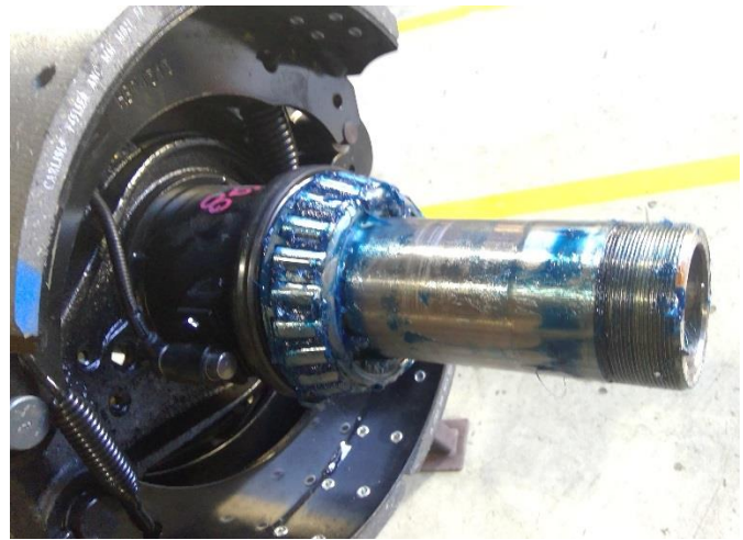
Photo showing a greased bearing fitted on to a greased spindle
