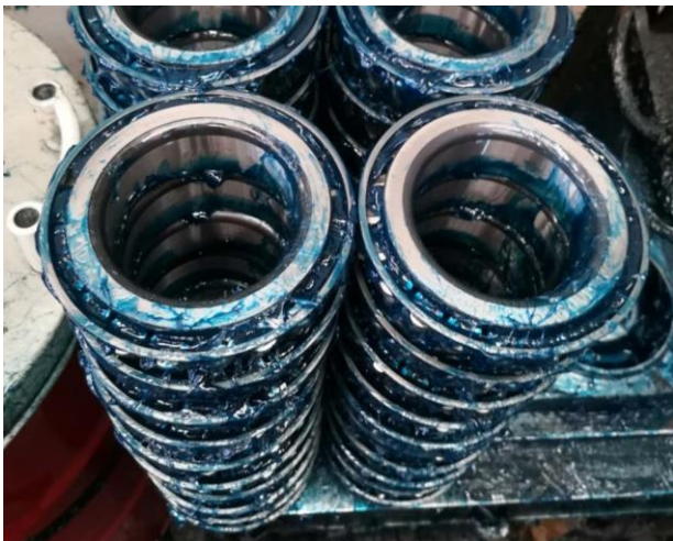
Photo showing the bearings packed with grease
