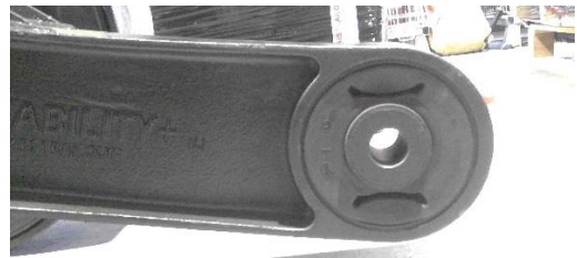
Photo showing the orientation of the pivot bush after installation
