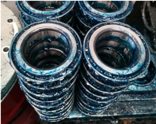
Photo showing the bearings packed with grease
