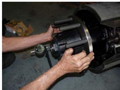
Push the hub and set the dial gauge to zero
