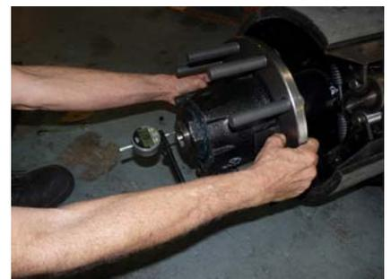
Pull the hub and check the reading
